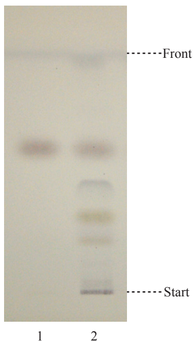
Figure 5 A reference HPTLC chromatogram of Myristicae Semen extract observed under visible light after staining
