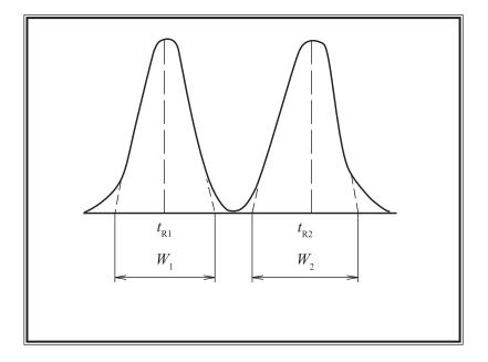
Figure 1 Parameters for calculation of resolution factor (R)
