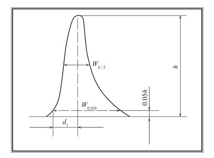
Figure 2 Parameters for calculation of tailing factor (T)
