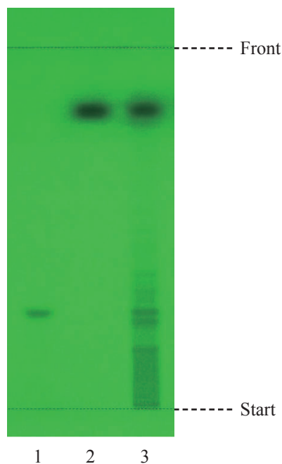
Figure 5 A reference HPTLC chromatogram of Citri Exocarpium Rubrum extract observed under UV light (254 nm)
