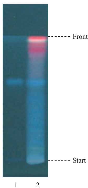
Figure 5 A reference HPTLC chromatogram of Centipedae Herba extract observed under UV light (366 nm)
