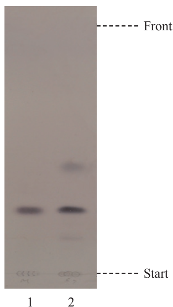
Figure 5 A reference HPTLC chromatogram of Ricini Semen extract observed under visible light after staining
