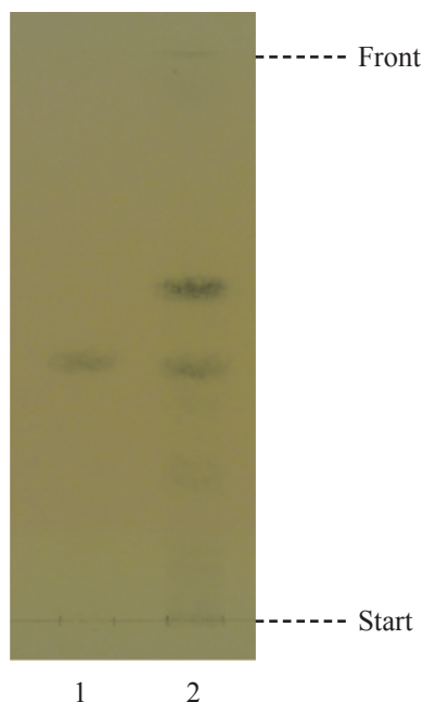
Figure 4 A reference HPTLC chromatogram of Buddlejæ Flos extract observed under visible light after staining
