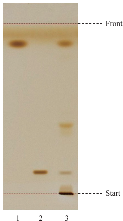
Figure 5 A reference HPTLC chromatogram of Arecae Semen extract observed under visible light after staining
