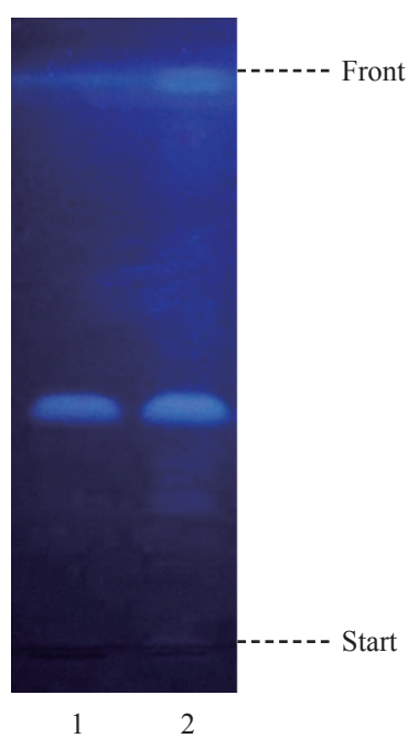
Figure 5 A reference HPTLC chromatogram of Allii Tuberosi Semen extract observed under UV light (366 nm) after staining
